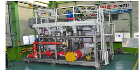
Partial Re-liquefaction System
