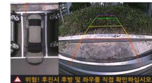
Ez Parking uses one (rear) or two (front and rear) cameras mounted on the vehicle to show the floor of the vehicle as well as the top view of the vehicle when moving the
