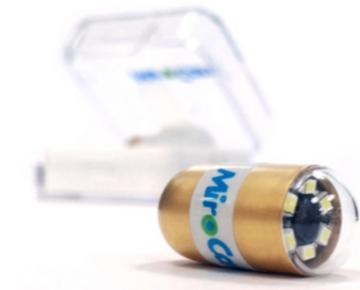
capsule captures images of the GI tract, which are sent via Human Body Communication to sensor pads which are affixed to the patient body. The sensor pads are connected to the receiver by the data cables. The image data is stored on the receiver for the duration of the patient procedure. After removing the receiver set from the patient body, the receiver is connected via USB to the Commercial PC and the image data is uploaded.
