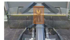
The transparent bucket is a safety assistance system that provides an image of the back of the bucket that blocks the driver's view. A never-before-seen concept,
