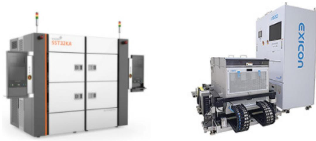
Storage Tester performs final SSD inspections using a number of different methods. Thus, by providing an equal testing environment through precision temperature control, this product helps determine faults in SSD products and inspects their performance and reliability.
